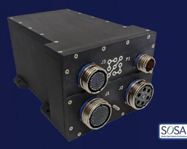
Helios is a rugged COTS vision computing system optimised for Size, Weight, Power and Cost (SWaP-C) and designed to operate in harsh environments.
