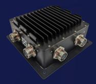
Hermod is a rugged Commercial Off the Shelf (COTS) Gigabit Ethernet switch optimised for Size, Weight, Power and Cost (SWaP-C) harsh environment embedded computer network applications.
