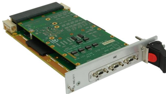
Air-cooled variant: 8 x Serial Communication Ports
