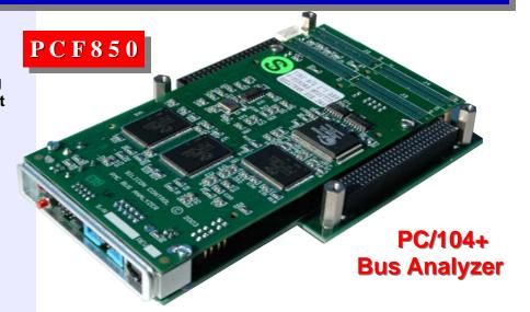
The PCF850 analyzes and exercises the 32 bit PCI bus in PC/104+ systems running at 0 to 133 Mhz. Over 100 protocol and timing violations are automatically checked and correlated with captured bus activity. System performance measurements include Bus Utilization, Transfer Rates, Latency, and Statistics.
